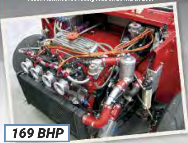
Stage 5 - (5 port) Cylinder Head 37.5mm inlets & 31mm exhaust valves
